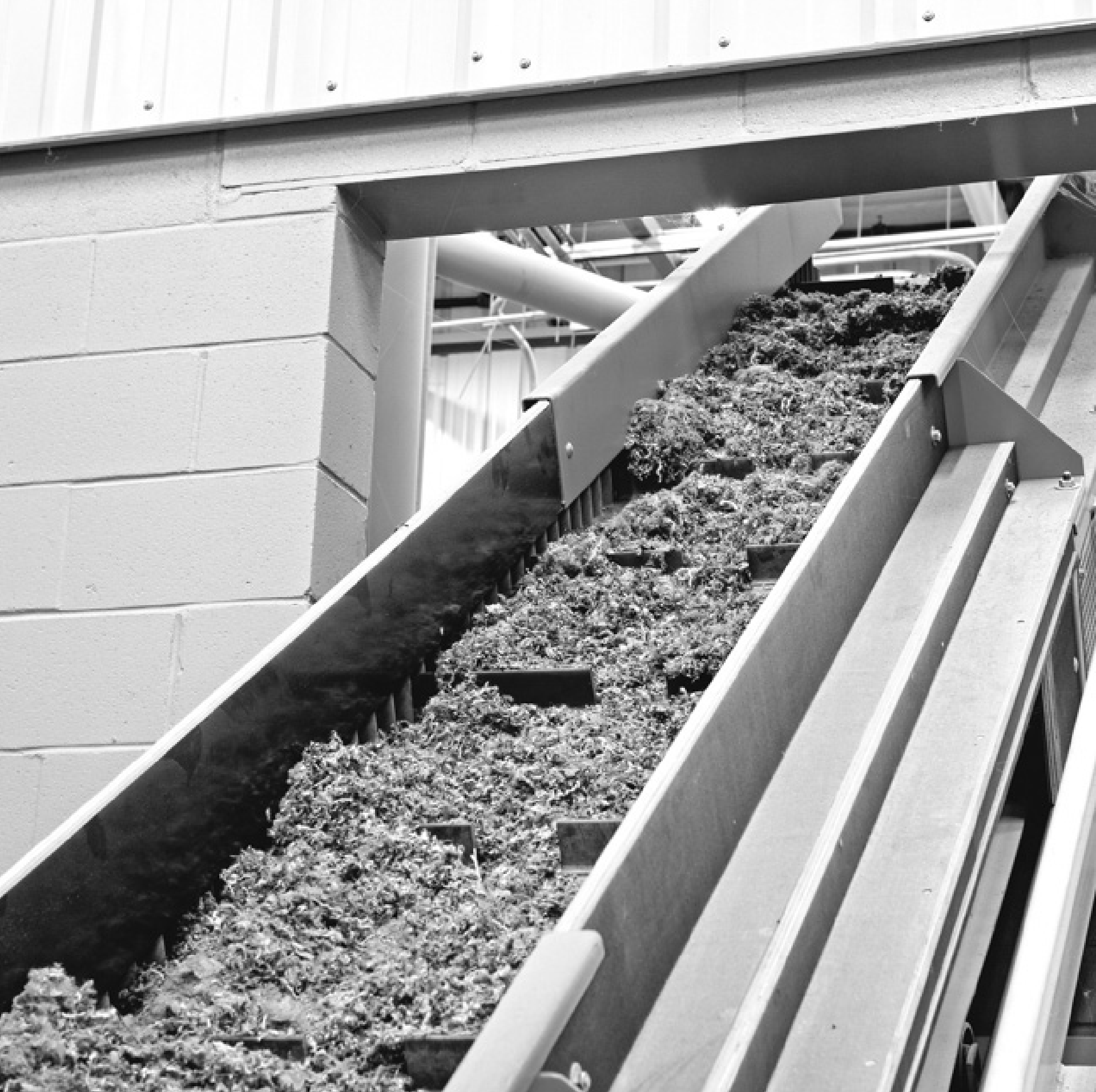
Separated GlasBac® and similar competitive backing is shredded and loaded into the agglomerator.
